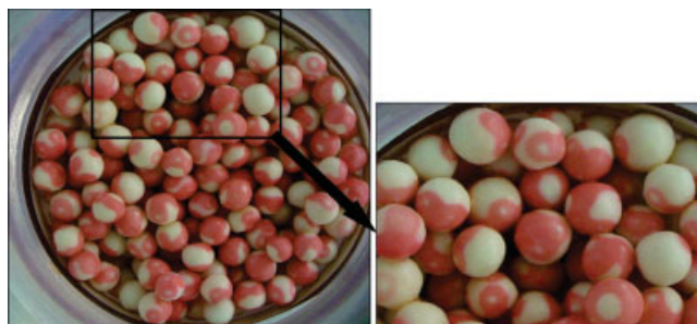
Figure 11. Picture of a column cross-section (pellets A; V_{LS} = 2 \times 10^{-3} m/s; water).
